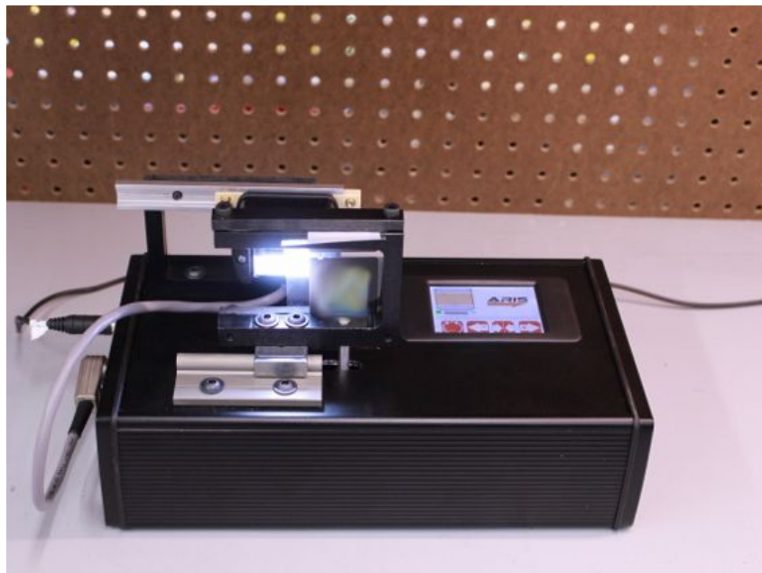
Fig. 2: High precision motor stage with a c-shaped fixture to hold the web material. A sensor mount with an option to mount 16 mm and 48 mm sensor at a working distance of 10 mm or 20 mm.
