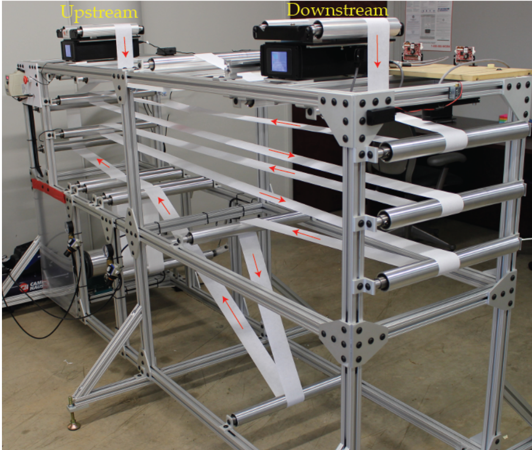
Fig. 2: The Experimental roll-to-roll machine used for testing the web guides.
