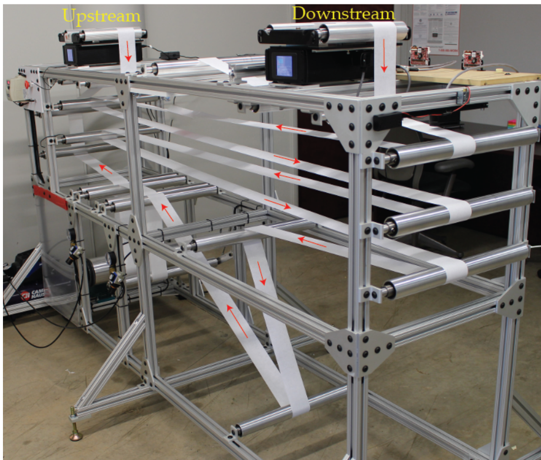
Fig. 1: The Experimental roll-to-roll machine used for testing the web guides.
