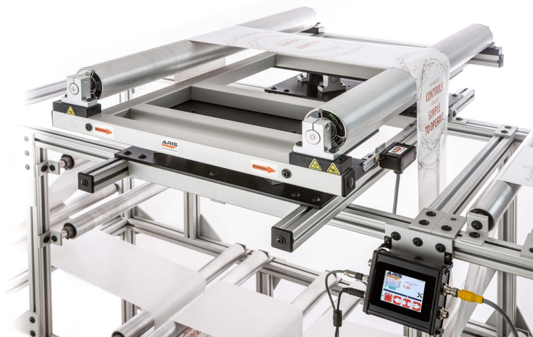
Fig. 1: Components of a web guiding system
