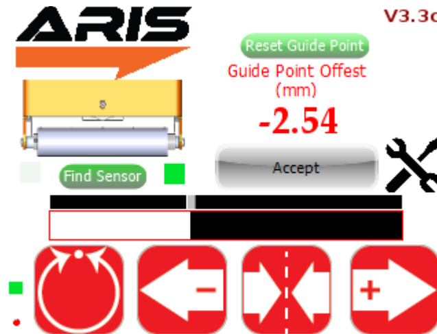
Fig. 8: Gross guide point adjustment
