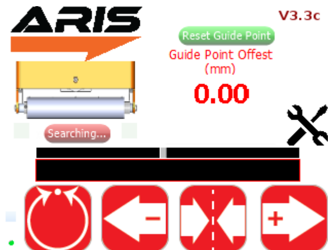
Fig. 12: Find sensor operation
