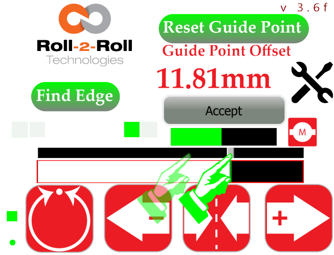
Figure 5.29: Release of track bar will prompt confirmation of the new guide point offset
